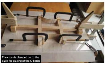
7 I clamp the cross on to my plate at the top- and bottom-block. Now I can bend the C-bouts with the drawing as reference. I mark their exact position in relation to the blocks, and glue them in with the clamps directly on the blocks' back edges. After setting these four clamps, I release the cross from the plate so that I can wash away any excess glue on the ribs and blocks, and the acrylic glass.
