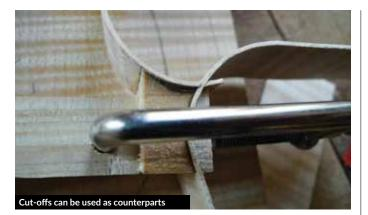
6 If I want to be really fast (when making a fractionalsized instrument, for instance), I simply cut out the block curves with a bandsaw and smooth them with a rasp. The cut-offs can be used as counterparts for the gluing.
