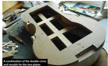
O This cross can be used for many other outlines. If I want to have more support for the outline (as when I'm making a cello, or using different outlines for the top and back) I cut out two moulds for the two plates and screw them on to the cross. Before gluing in the linings I unscrew them.
