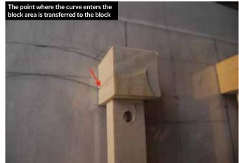
5 When shaping the blocks, the important areas are the curves at their ends, as they determine the direction of the ribs when leaving the blocks. To control them I transfer their position from the drawing on to the blocks with a ruler. This also gives me the reference points to lay out the corner templates. (For a looser approach I can skip this step or deliberately displace or rotate the template a little.) >
