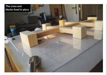
I plane the blocks to the dimensions (length and width) shown on the drawing. Then I draw a centre line on the top- and bottom-blocks and the cross to mark their positions. Since the cross is thinner than the blocks, it needs to be supported. (I generally place a CD case under the cross for this.) Then I fix the blocks in place with white glue. I begin with the upper and lower bout, then I set the cross on the
